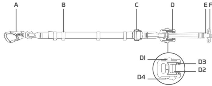
**A** Connector for the anchor point | **B** Elastic loops | **C** Length adjustment buckle | **D** Quick-release device | **D1** Safety sleeves | **D2** Insert | **D3** Red marking points | **D4** Release buttons | **E** Eyelet for connection to the harness | **F** Fast-Rubber
