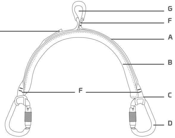
A Polyamide lanyard | B Aluminium alloy spacer | C Fast-Rubber | D Connectors compliant with EN 362 | E Main seam | F Secondary seam | G Suspension connector loop
