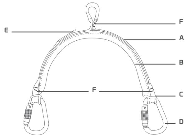
**A** Polyamide lanyard | **B** Aluminium alloy spacer | **C** Fast-Rubber | **D** Connectors compliant with EN 362 | **E** Main seam | **F** Secondary seam
