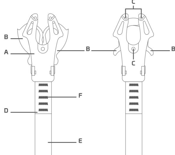
A Body | B Gates | C Pins | D Sling | E Eyelet | F Stitch
